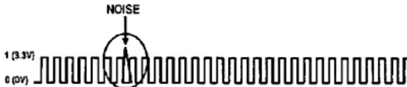
Figure 2. High Frequency Noise From, 50MHz, 3.3 Volt
