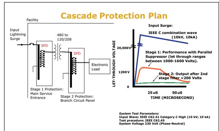
Figure 2. In this graph, the blue line is a surge without any protection. Note that the voltage level exceeds 20,000 V. The red line is a surge with one SPD installed. Note that the voltage level still exceeds 1,200 V, which can cause damage. The green line is what remains of the initial surge with two SPD devices installed.
